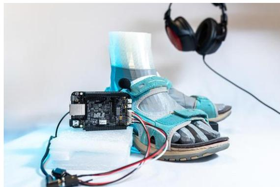
Figure 3 - Complete test system with the Bela.io implementation.
